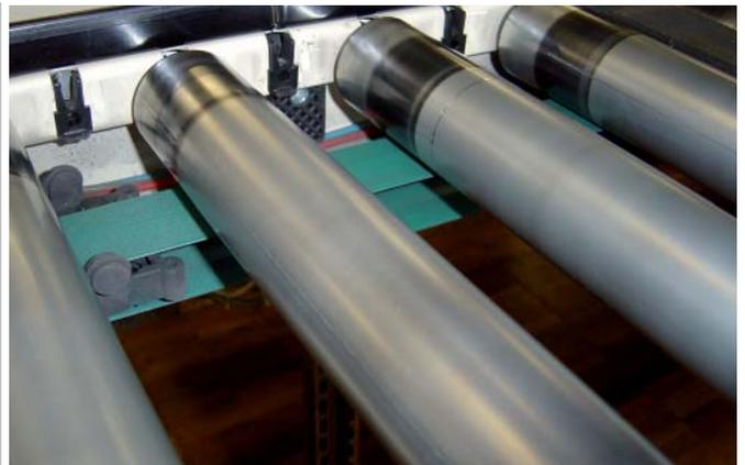
Flat belt driven LRC are particularly well suited for goods accumulation and subsequent singulation processes. For the selection of the flat belt it is important to know exactly which LRC system will be used.
