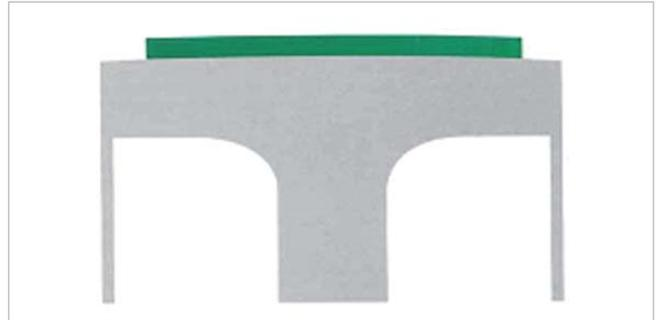
Frictional engagement on the outer pulley surface require only a small cross-section and make flat belts very flexible
